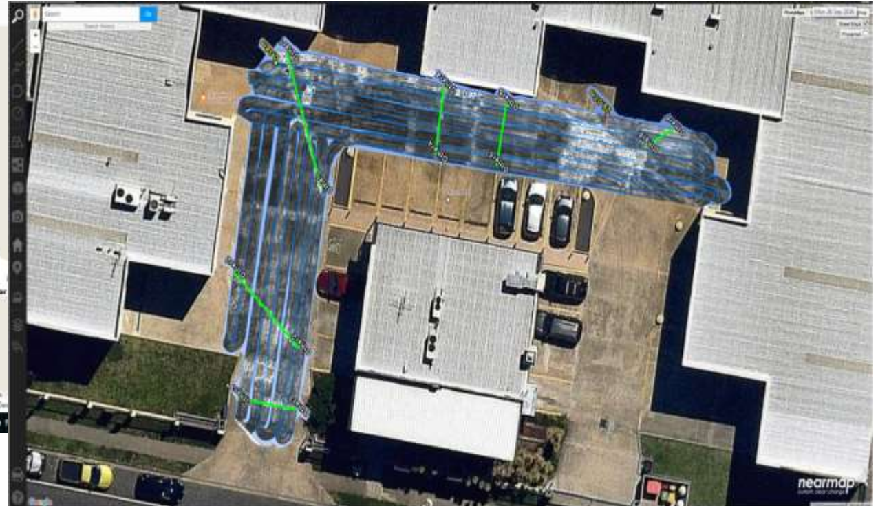
On site visualization of detected pipes on imported cartography and images
