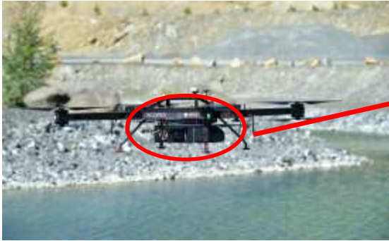
BathyCopter with RIEGL BDF-1 sensor payload
