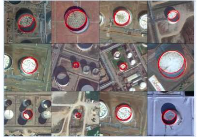
Each new image acquired over the areas are processed to measure the fill percentage (97% accuracy)
