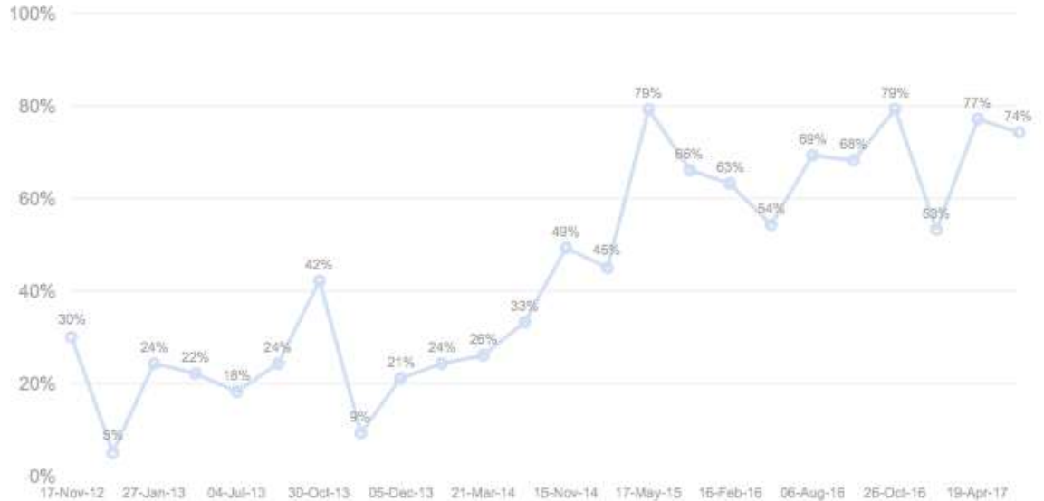
Crude oil fill percentage evolution over a group of 8 tanks during a 5 year period
