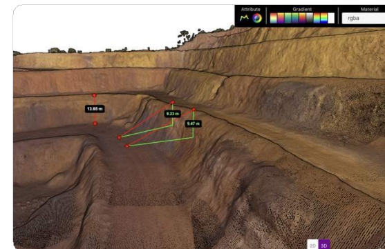
Haul road slope measurement
