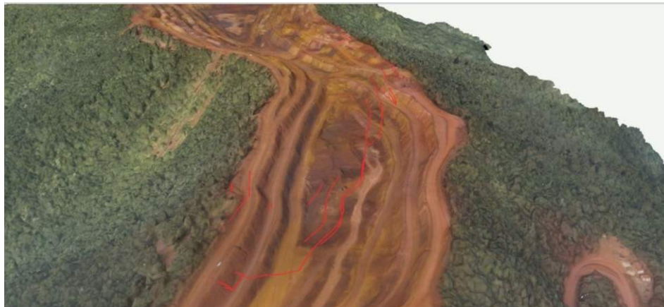
3D model visualization of large scale data with plan (KML) overlay
