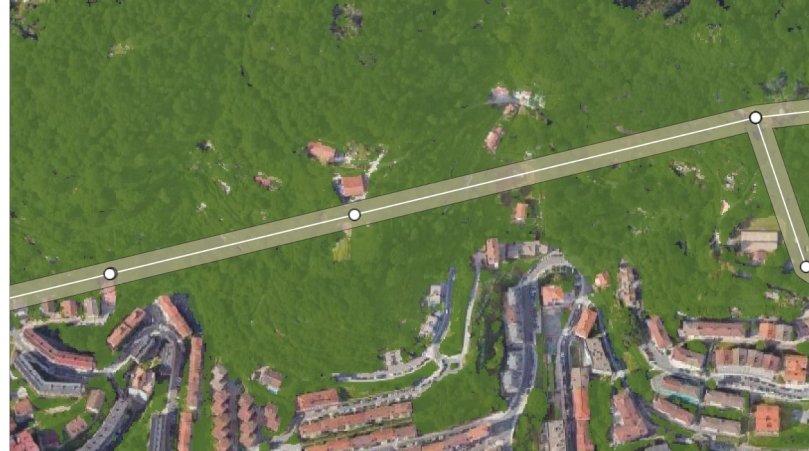
The vegetation mask algorithm is implemented on the hi-res satellite images for detecting vegetation in and around the ROW of the power line
