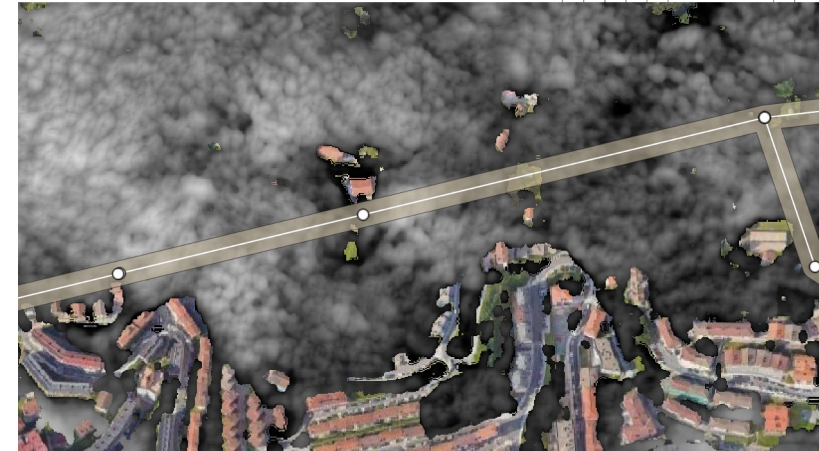
Using stereo pair satellite images, height of the vegetation is determined
