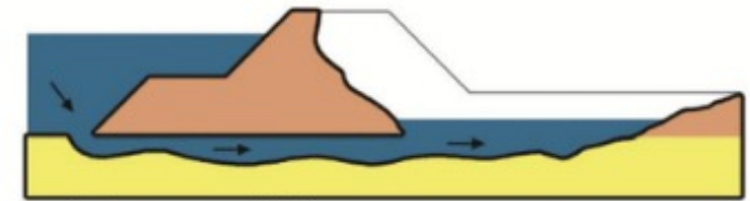
e) Levee failure
