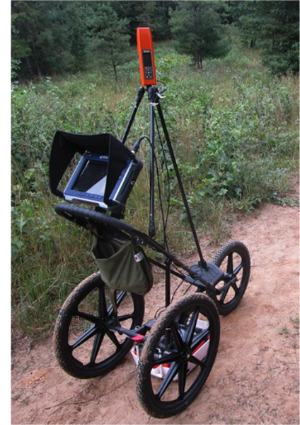
Ground Penetrating Radar (GPR)
