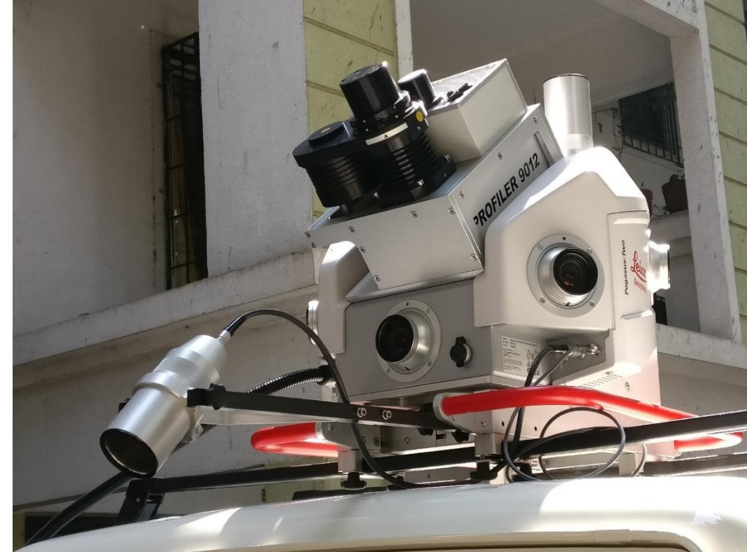
Network Survey Vehicle (NSV) : 'Leica Pegasus Two' with pavement Camera
