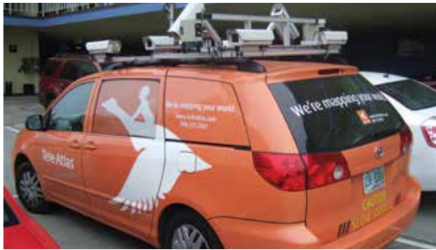
The Tele Atlas mapper van had cameras on the top and the hard drives cabinet in the customized rear seat. Since July 30, 2008, the company has been a wholly owned subsidiary of automotive navigation system manufacturer TomTom
