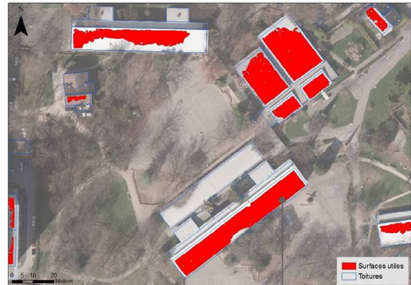
Useful roof surfaces
