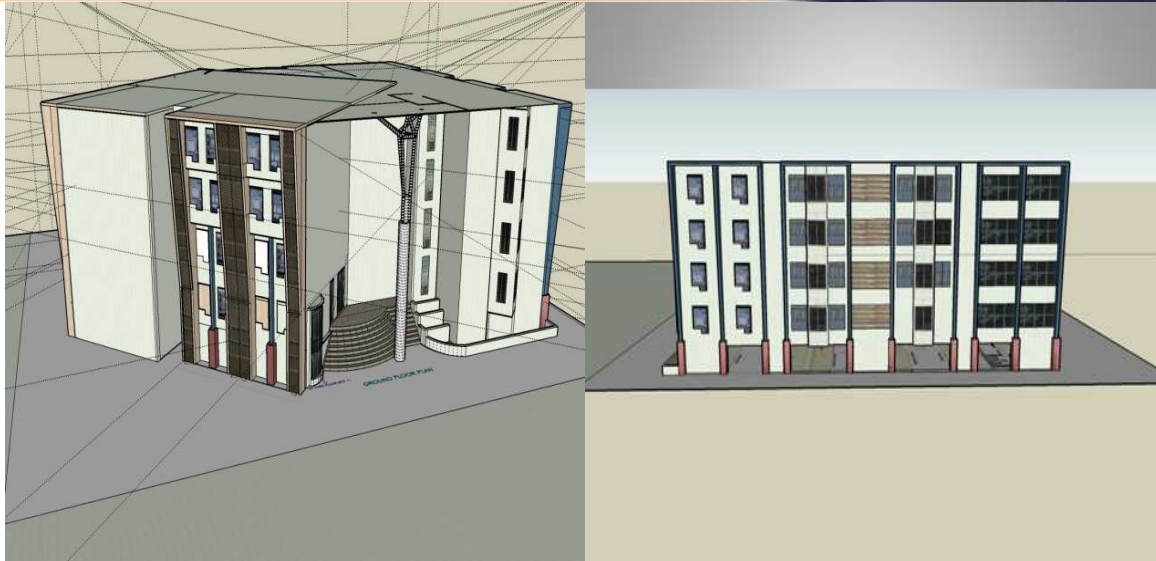
Fig.8: LoD2 model of the KRESIT Building, created and visualized in Google SketchUp.
